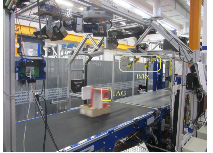
Fig. 4. Luggage sorting on a conveyor belt using UWB-RFID tags [25].
