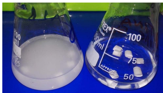
Fig. 7. Effect on cement pastes cohesion of 0.5% of AL directly dispersed into the starting powders (left) and loaded with -MPs-Cut-AL (right).
