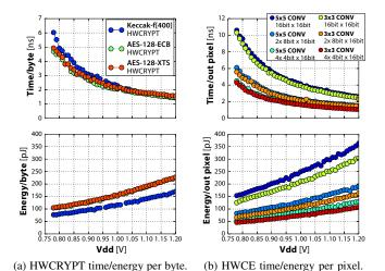
Fig. 6: Performance and efficiency of the HWCRYPT and HWCE accelerators in terms of time/energy for elementary output.
