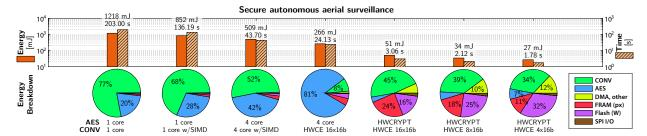
Fig. 8: Secure autonomous aerial surveillance use case based on a *ResNet-20* CNN [10] with AES-128-XTS encryption for all weights and partial results. KEC-CNN-SW and CRY-CNN-SW operating modes at  $V_{DD} = 0.8 \,\mathrm{V}$ .
