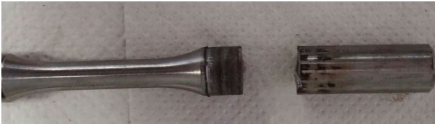
Figure 4: Unexpected failure at sample head
