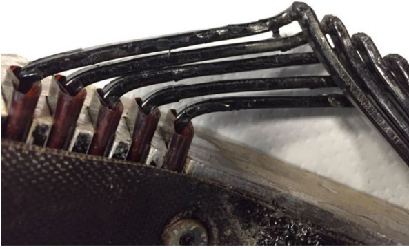
Fig. 5. End winding of the formette after 15 aging subcycles at 250 °C.
