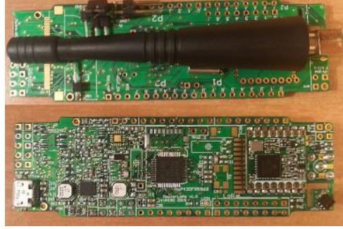
Fig. 5. Prototypes of the wireless module with LoRa transceiver.
