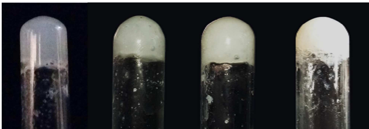
Figure S1. Photographs of samples of hydrogels 2 , 3 , 4 and 6 prepared with gelators A , B and C and of hydrogels obtained with the gelators A-C and a stoichiometric amount of \text{CaCl}_2 . Hydrogels 1 and 5 were not included because they are partial gels (see Table S1 for details).
