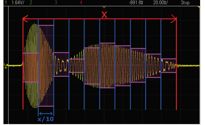
Fig. 4. General description of the discrete sum used for calculating the area of the waveform for power estimation
