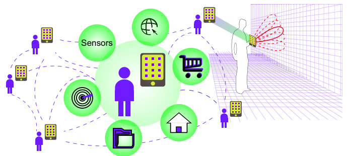
Fig. 1: Users, equipped with massive arrays on their smartphones, in participatory or not manner scan indoor environments with the opportunity to share their maps.
