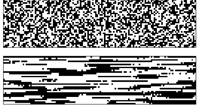
Fig. 2: An antipodal sensing matrix following standard CS (top) coupled with another antipodal sensing matrix generated as prescribed by the rakeness-based CS for ECG signals (bottom). Both matrices were generated with CR=4 . Note that white means -1 while black corresponds to +1 .
