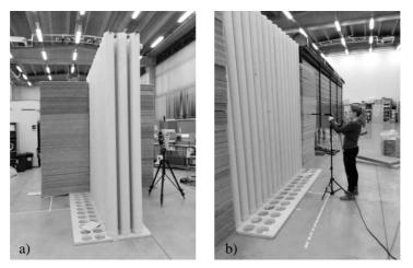
Figure 7 - Misure intensimetriche sul lato (a) e sul retro (b) del cristallo sonico -Sound intensity measurement setup on the side (a) and the rear (b) of the sonic crystal.
