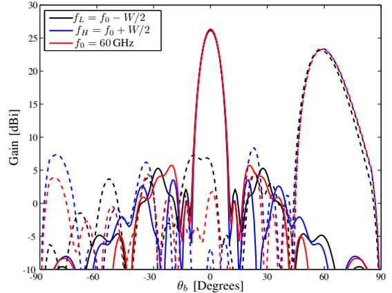
Fig. 4. Theoretical gain of 2-bit  $15 \times 15$  TA as a function of the steering angle  $\theta_b$  with  $W = 1$  GHz and for  $(F/D)_{\text{opt}}$  ratio. Continuous lines refers to the case  $\theta_b = 0^\circ$ , dashed lines refers to the case  $\theta_b = 60^\circ$
