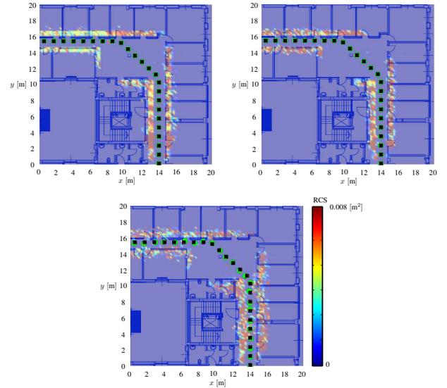
Fig. 6. Mapping results using  $15 \times 15$  TA with a perfect knowledge of TA-radar position and orientation and with a reduced focal distance  $F = 10\text{mm}$  (top-left) and  $F = 5\text{mm}$  (top-right), and with TA-radar position and orientation errors and  $F = 10\text{mm}$  (bottom).
