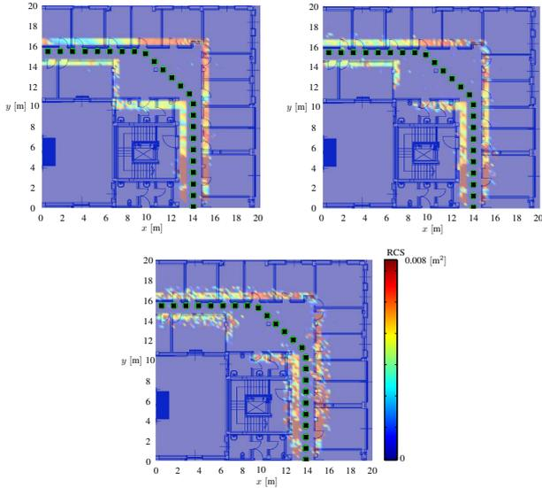
Fig. 5. Mapping results using  $20 \times 20$  (top-left),  $15 \times 15$  (top-right) and  $10 \times 10$  transmitarray (bottom) with 2 bits phase compensation, optimal  $F/D$  ratio and with a perfect knowledge of TA-radar position and orientation.
