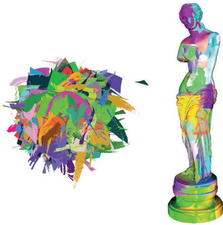
Figure 10: Registration of the Venus de Milo by alignment of 61 views and about 50 million points.
