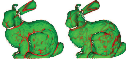
Figure 5: Flatness Vs Orientability. On the left the flatness map of a view, on the right the corresponding orientability map. The green colour represent flat and highly-orientable points respectively, red points feature high curvature in the flatness map and poor LRF repeatability in the orientability map.
