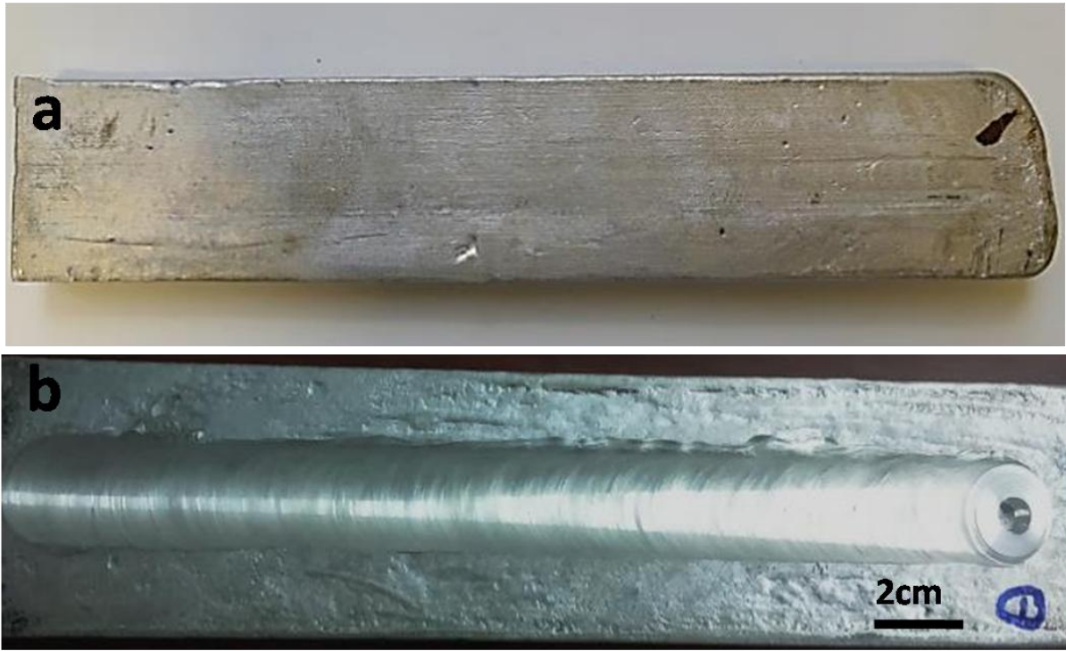
Figure 1. Macrographs of AA2024-Al 2 O 3 nanocomposite in the (a) as cast condition and (b) after FSP.
