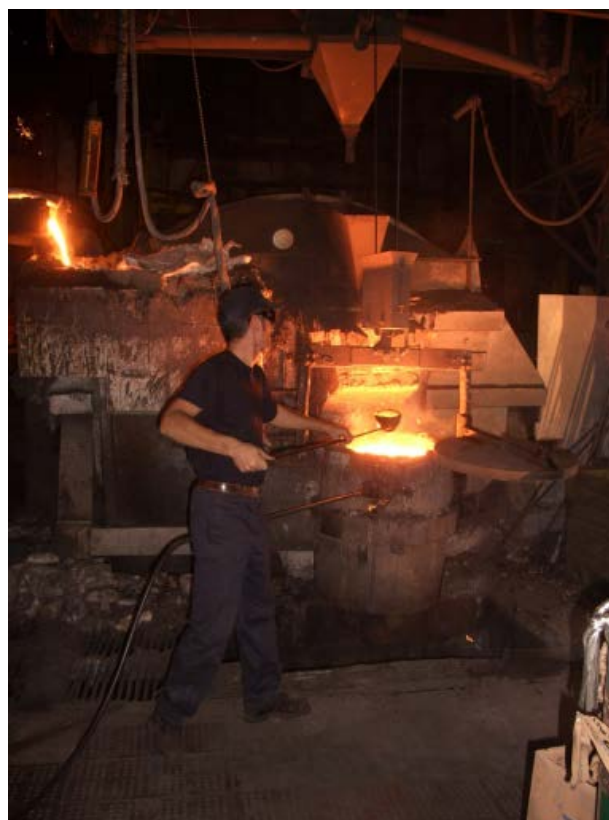
Fig. 4. Sample taking from ladle permitting a thermal analysis with the aim at obtaining the chemical composition of alloy after the inoculation of additives (Courtesy SCM Group).
