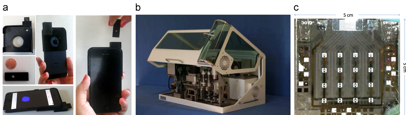
Fig. 1. Different platforms for CL detection. (a) The accessories (minicartridge and smartphone adapter) and their integration with the smartphone for point-of-need-analysis based on chemical luminescence detection (Roda et al., 2014b), Copyright 2014, reprinted with permission from American Chemical Society. (b) The MCR3 instrument for microarray analysis (Seidel and Niessner, 2014), Copyright 2014, reprinted with permission from Springer. (c) The a-Si:H photodiodes array (Mirasoli et al., 2014a).
