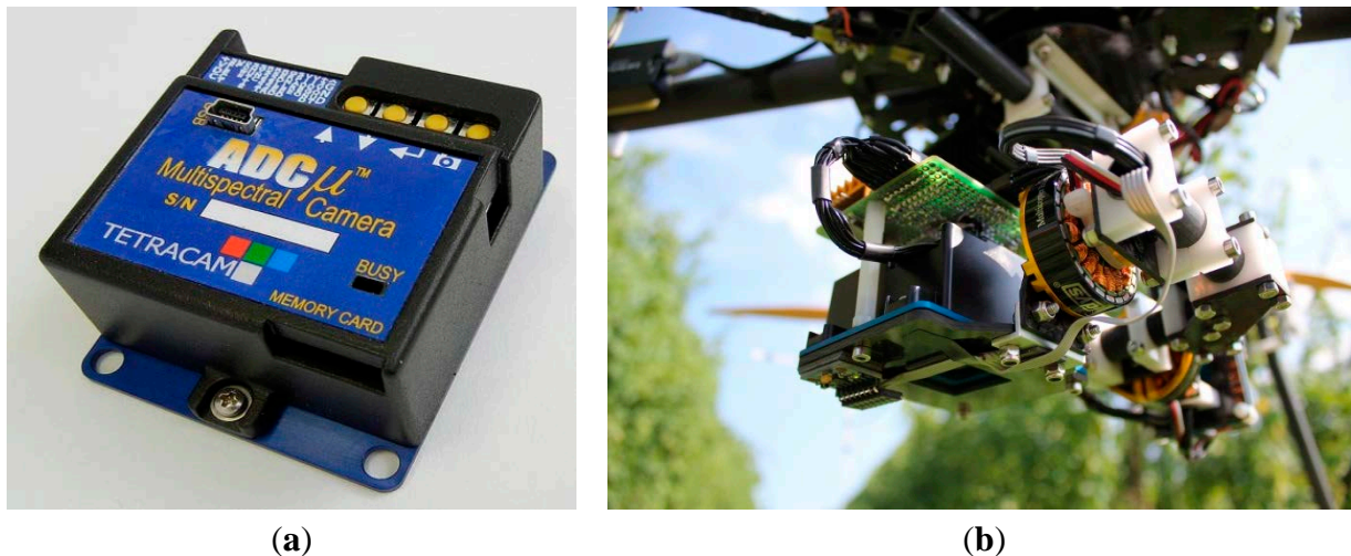
Figure 4. The multispectral camera TETRACAM ADC Micro (a). The tested multispectral gimbal (b).
