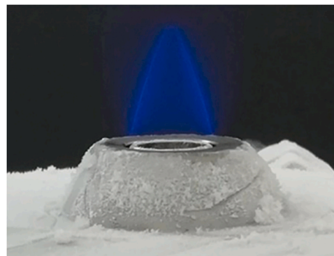
Fig. 4. Example of methane–air flame at a temperature of 230 K, captured with a Digital Single-Lens Reflex camera. Adapted from (Ghosh et al., 2022a).
