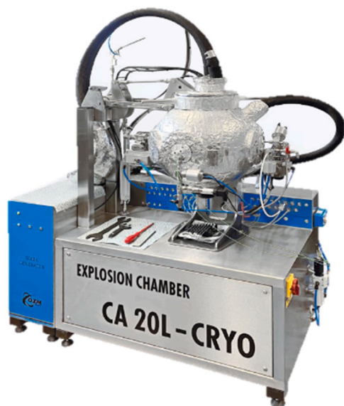
Fig. 12. Explosion chamber for gases, vapors, and dusts, approx. 20 L (CRYO version) (OZM Research s.r.o., 2025).
