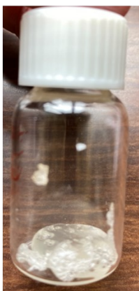
Figure S2. a) Typical appearance of the poly(vinyl acetate- co -crotonic acid) polymer obtained from the raw product after precipitation in cyclohexane; b) Poly(vinyl acetate- co -crotonic acid) polymer obtained upon irradiation of the mixture of monomers in the presence of different PIs. From left to right: with HCPK, BAPO, DMPA and CQ.
