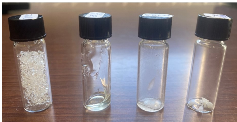
Figure S2. a) Typical appearance of the poly(vinyl acetate- co -crotonic acid) polymer obtained from the raw product after precipitation in cyclohexane; b) Poly(vinyl acetate- co -crotonic acid) polymer obtained upon irradiation of the mixture of monomers in the presence of different PIs. From left to right: with HCPK, BAPO, DMPA and CQ.
