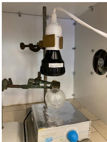
Figure S1. Irradiation set-up prior (left) and during (right) the irradiation of the mixture with the EvoluChem Lamp (18 W, emission centered at 405 nm).
