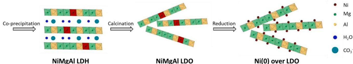
Fig. 1. Schematization of the NiMgAl hydrotalcite-derived catalyst preparation procedure.
