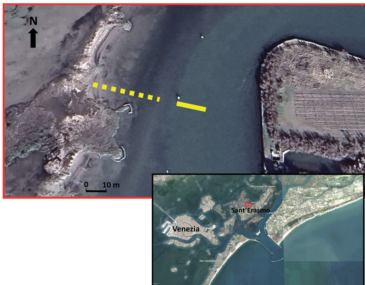
Fig. 3. Location of the survey area in the Venice lagoon and detail of the position of the embankment in the Passaora channel. The continuous yellow line indicates the section identified on the bottom of the channel, the dashed line its probable development towards the west, identified by means of metal probe survey and coring under the shallow area and under the sandbar (S.M. processing based on GoogleEarth).
