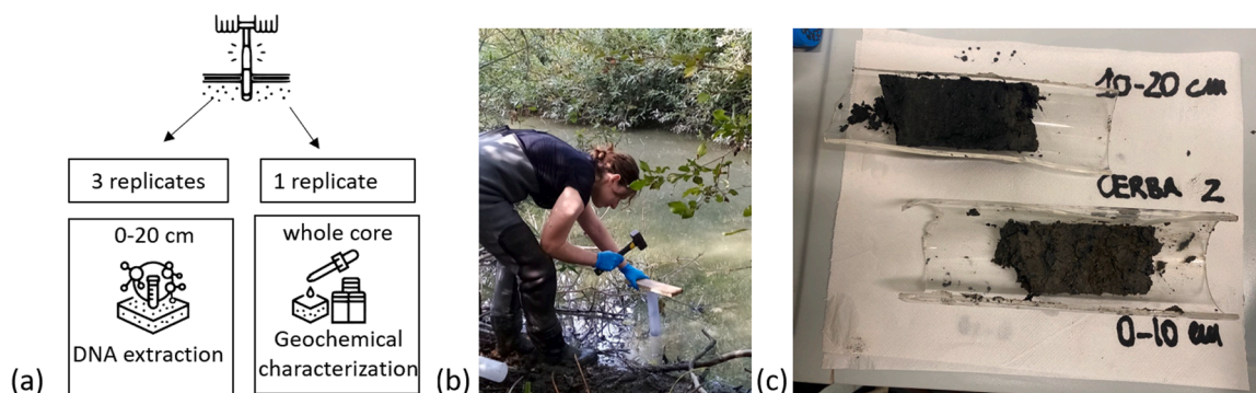
Fig. 2. (a) and (b) Sediment core sampling design at each sampling site using plexiglass tubes (a and b); (c) core sections at different depths extracted in the laboratory for microbial analysis.
