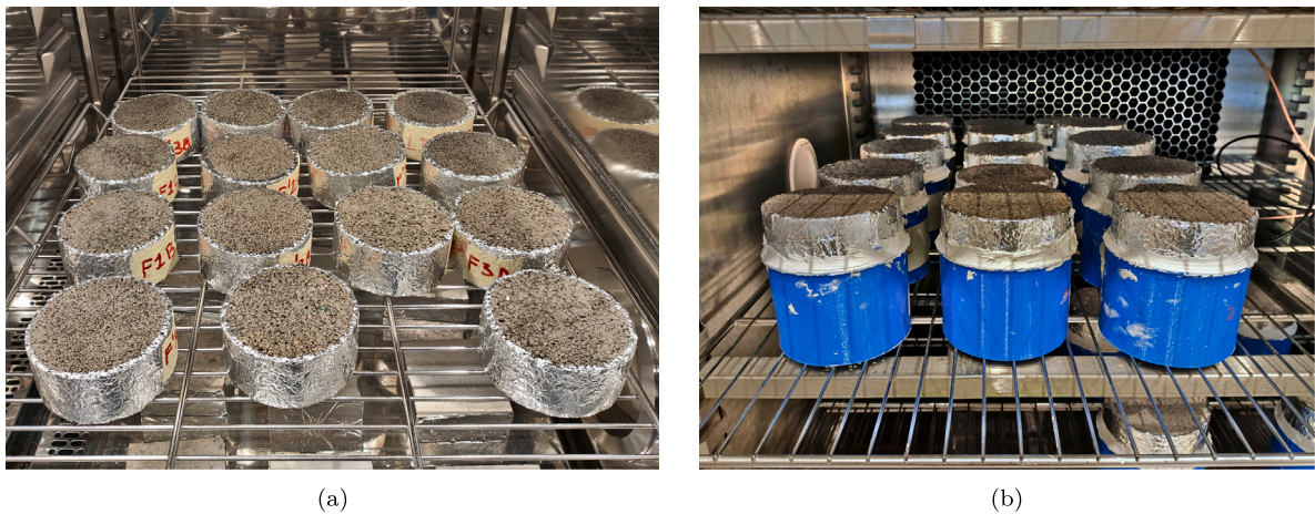
Fig. 5. Measurement of MBV and water vapor resistance, respectively through the NORTDEST protocol (a) and the wet cup method (b).
