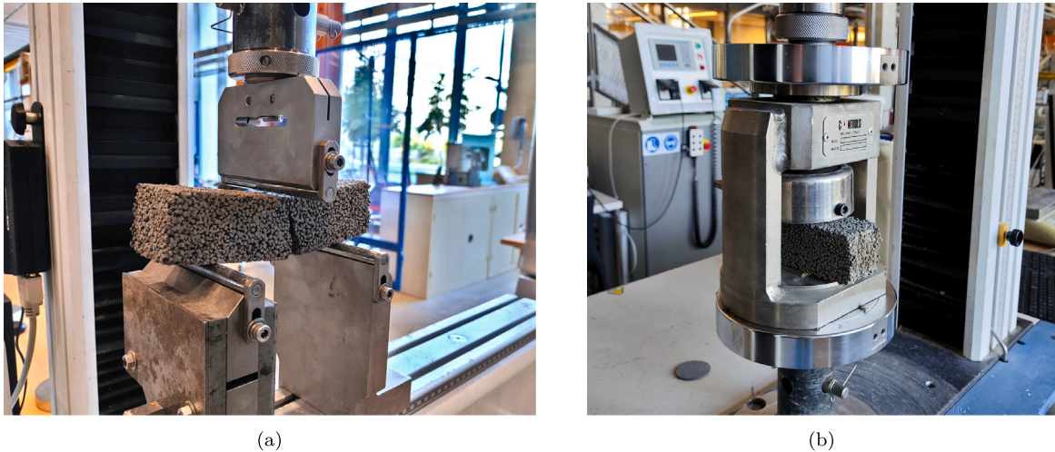
Fig. 3. Setups employed to carry out flexural (a) and compressive (b) tests.
