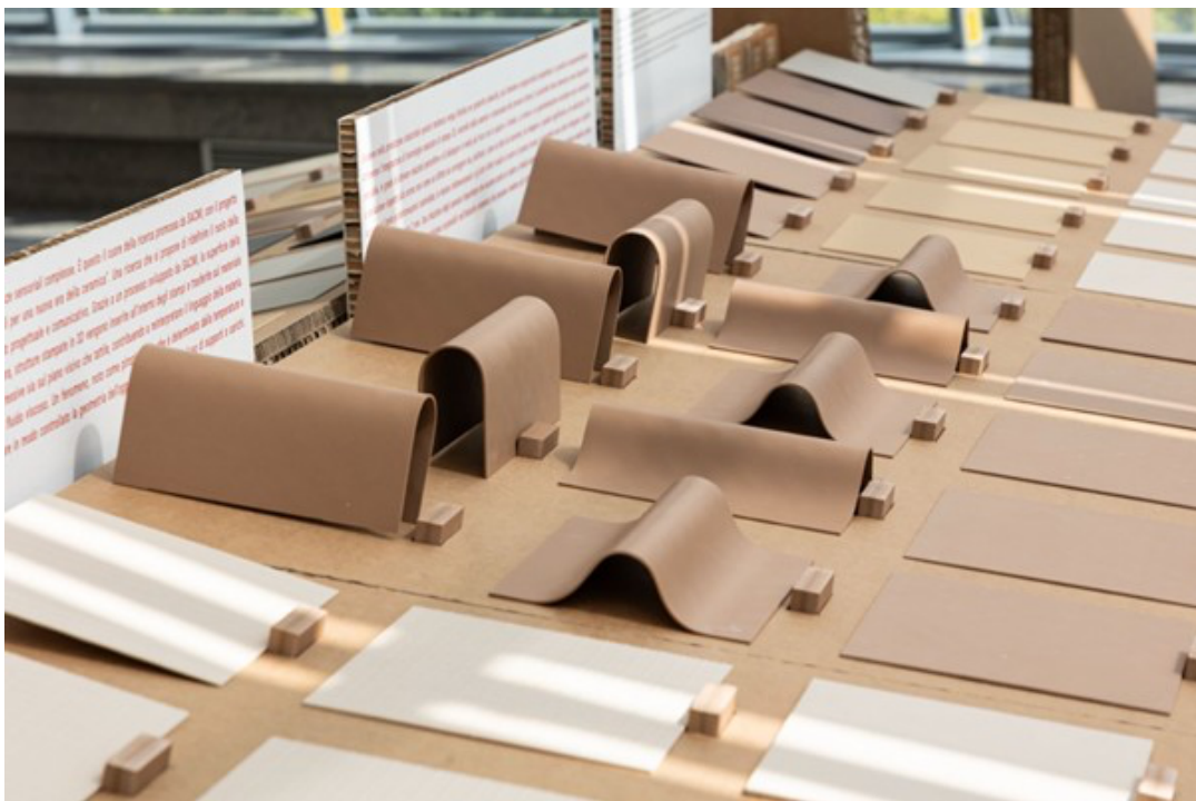
Fig. 3 Bending and deformation experiments. Mechanical stress tests demonstrating how the material can support non-conventional geometries and fabrication strategies. Image source: MICS Foundation
