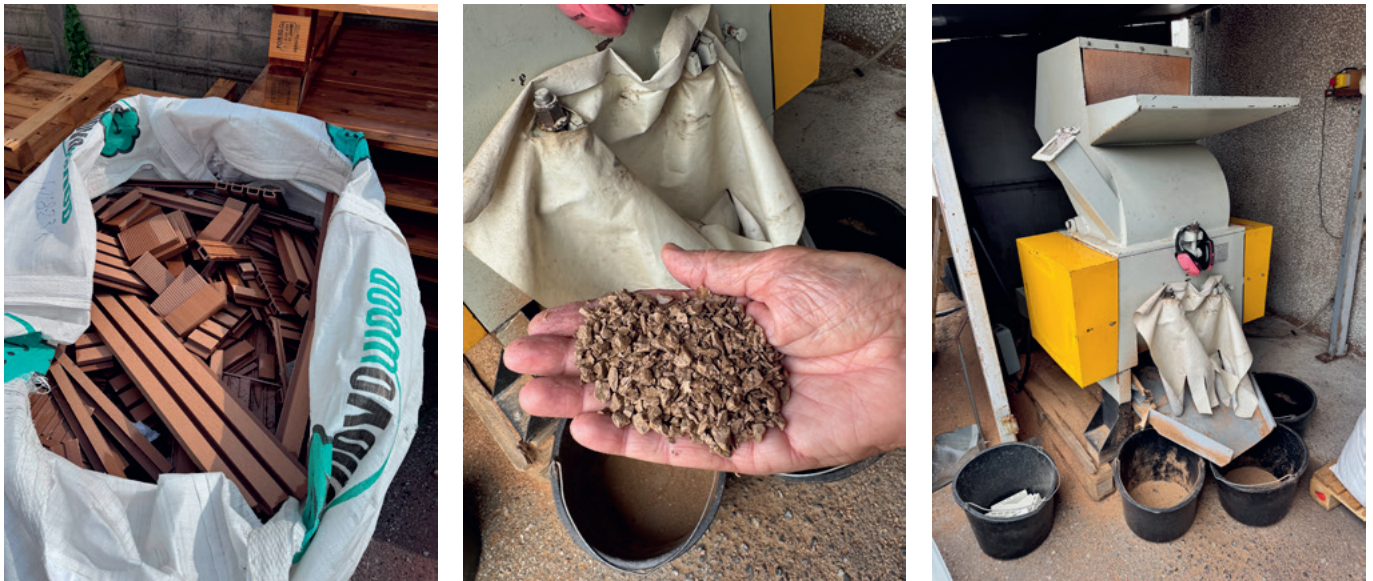
Fig. 6. (From left to right) Big bag containing the site scraps; Shredded WPC; Shredding machine. © 2025, Iperwood®.
