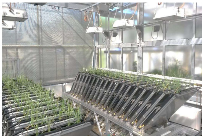
FIGURE 1 GROWSCREEN-Rhizo rhizoboxes and wheat genotypes in the high-throughput phenotyping platform (HTPP).
