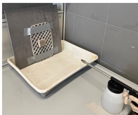
Figure 2: Experimental setup for the application of artificial rain.
