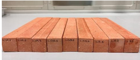
Fig 3. Brick samples selected for the experiment ( 3 \times 3 \times 25 \text{ cm}^3 )
