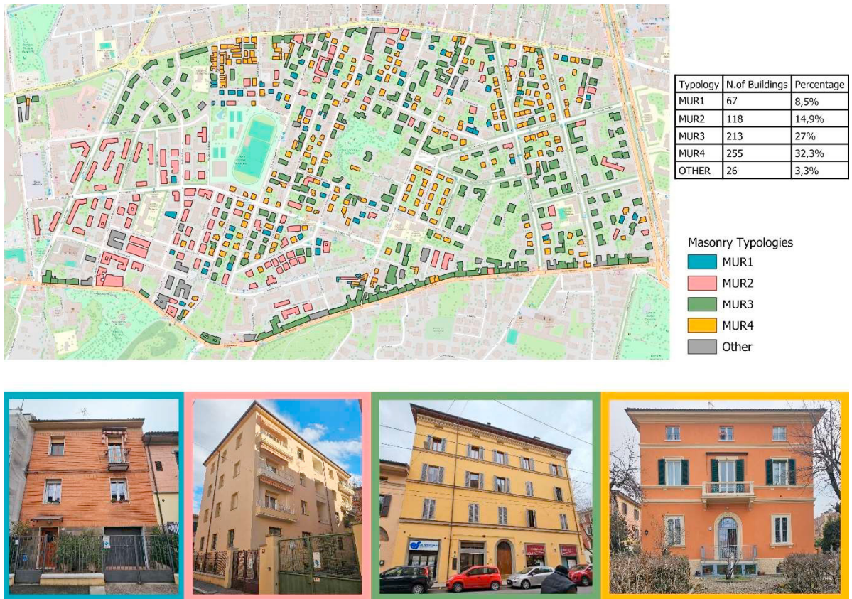
Fig. 5. Masonry building typologies in the Saragozza district (percentages are referred to the total number of residential buildings).
