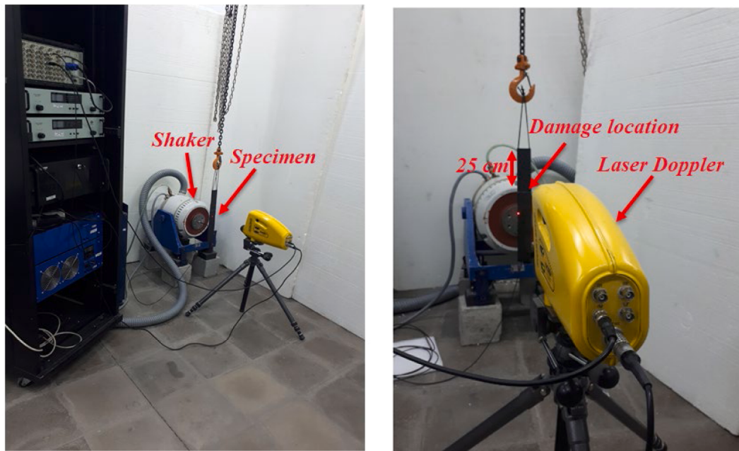
Fig. 7. Experimental modal analysis setup used in the current study location of damage in the considered laminated composite beam.
