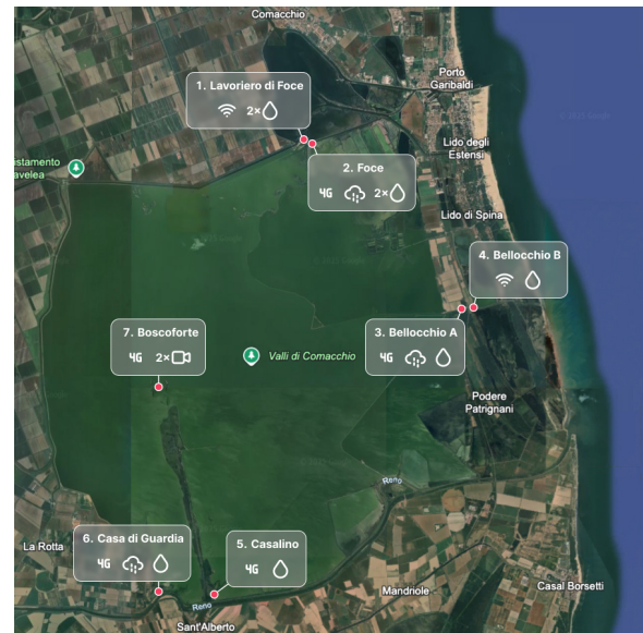
Figure 1: Map of the sensing infrastructure deployed in the Comacchio Lagoon, comprising six weather and water monitoring stations (stations 1-6) and one fauna monitoring station (station 7). Icons indicate the specific hardware components installed at each station.
