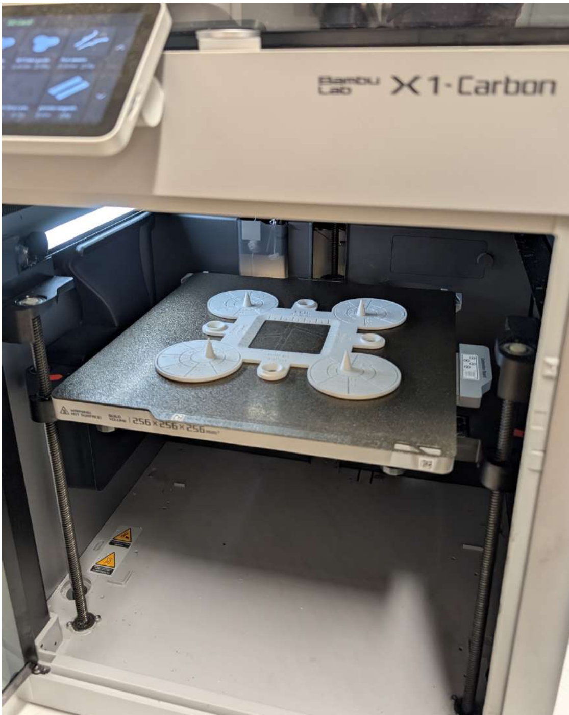
Fig. 2 The Shadow-Aided Light Alignment Frame (SALA- Frame) (Credits: 3D print and photo Gaeta B., SALA- Frame Foschi R., 2025).
