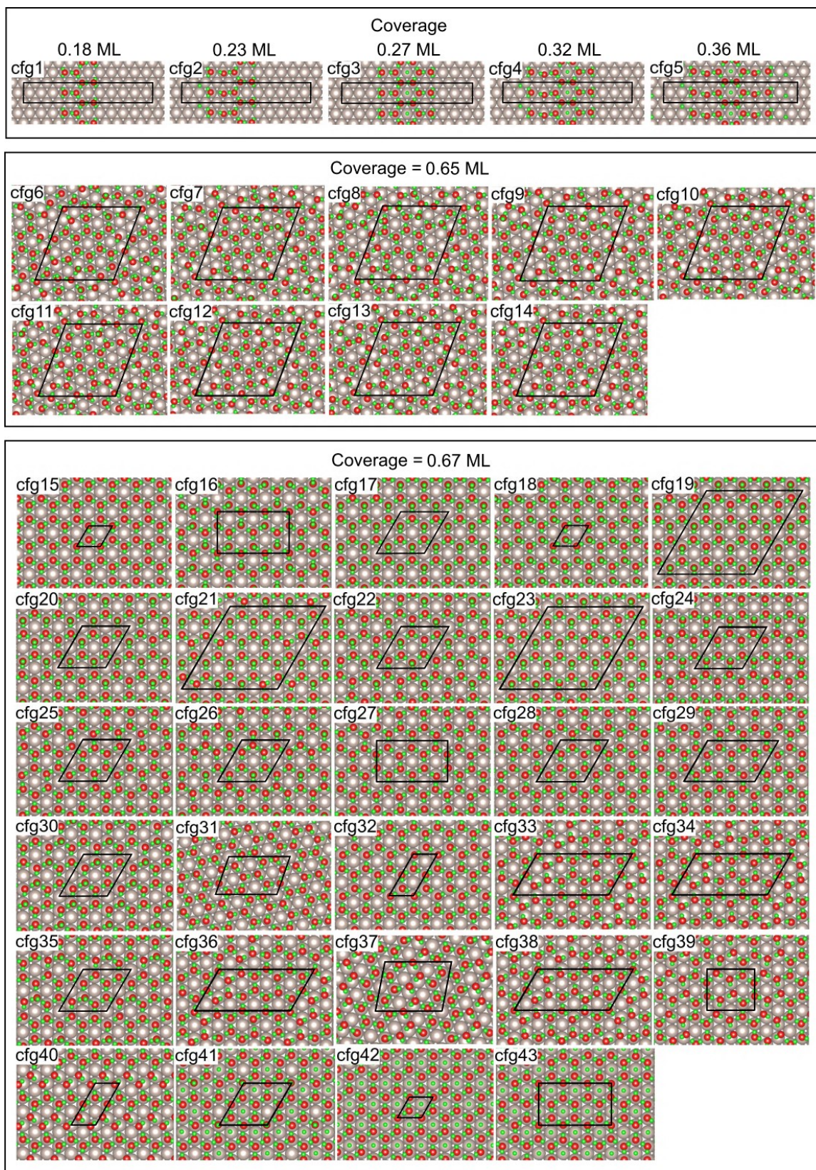
Figure S2. The considered 43 water overlayer configurations on Ru(0001) with various coverages, for which the adsorption energies were calculated and displayed in Figure 1 of the main text. The configurations from cfg1 to cfg4 were taken from Ref. [18]. The configuration cfg5 was extracted from Ref. [18, 19]. The configurations of cfg6-cfg14, cfg17, cfg19-cfg24, cfg26, cfg30, and cfg35 were taken from Ref. [20]. The configurations of cfg15, cfg16, cfg18, and cfg43 were extracted from Ref. [16]. The configuration of cfg32 was obtained from Ref. [17]. The configurations of cfg25, cfg27-cfg29, cfg31, cfg33-cfg34, and cfg36-cfg39 were derived from Ref. [8]. The configurations of cfg41 and cfg42 were obtained from Ref. [7]. The Ru, O, and H atoms are represented by brown, red, and green spheres, respectively. The black lines indicate the unit cell.
