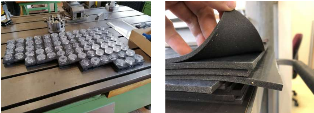
Figure 6. Left side: Mirrobor seals prepared to cover bolts and screws holes in the ColdBox. Right side: Mirrobor sheets before the machining process.
