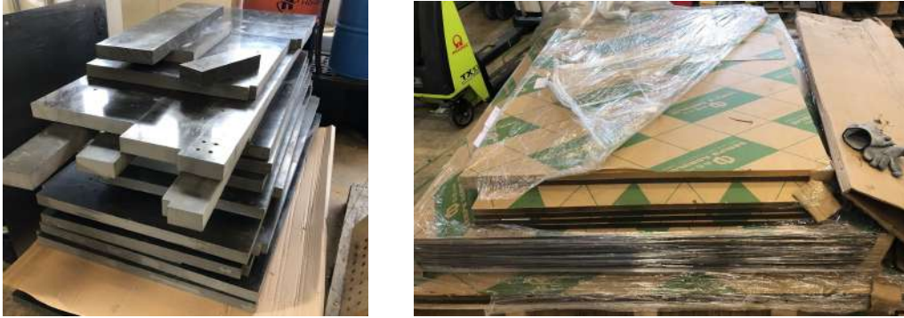
Figure 4. Left side: machined borated polyethylene. Right side: plexiglass sheets before the machining process.
