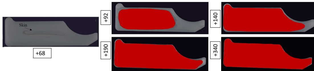
Figure 6 – Charge weld evolution Extrusion Case study D. Distances from the stop mark in [mm]. The experimental data obtained from [11].
