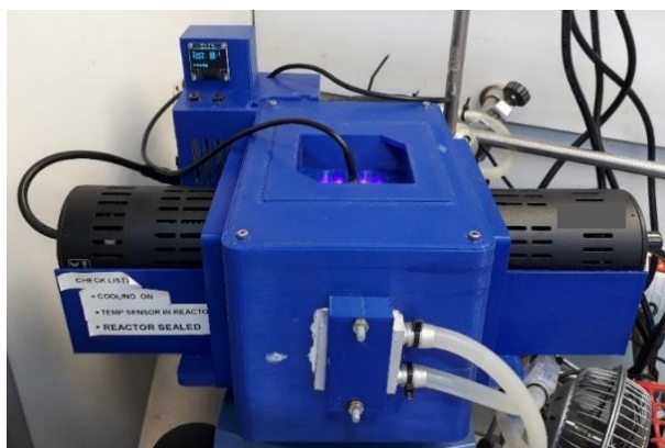
Figure S5. Reaction set-up for small-scale reactions using a 3D-printed, temperature controlled photoreactor, 3 illuminated at 390 nm with two Kessil PR160L lamps.
