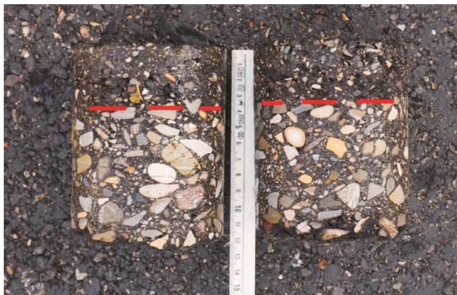
Fig. 5. Samples cored from the trial field with layers separation.
