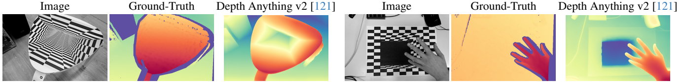
Figure 3. Samples from MonoTrap Dataset. We report two scenes featured in our dataset, showing the left image, the ground-truth depth, and the predictions by Depth Anything v2 [121], highlighting how it fails in the presence of visual illusions.
