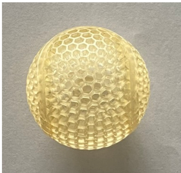
Fig. 5 A honeycomb-patterned hollow tennis ball printed with 75% PDHIA_0.5, thus containing 22 wt% recycled PET. Object diameter is 40 mm.
