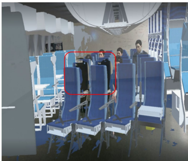
Fig. 4 Extended reality real-scale Flying-V model. Physical seats in the red square
