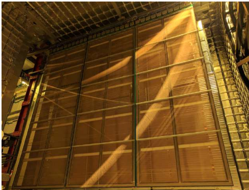
Figure 1. Three APAs in front of the field cage and cryostat wall. Repriduced from [5]. The Author(s). CC BY 4.0.
