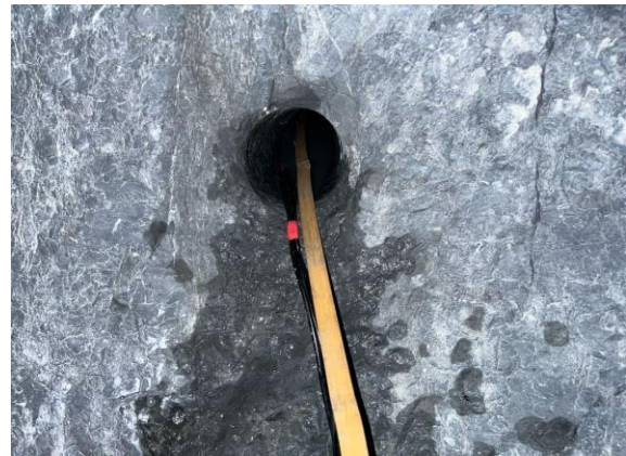
Fig. 6. Field acoustic wave testing
