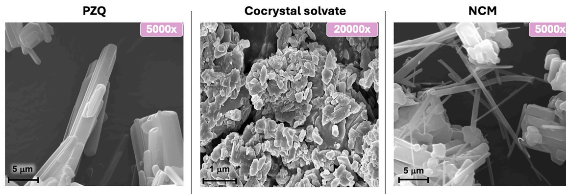
Fig. 10. SEM images of (a) PZQ (5000x), (b) PZQ-NCM-AA cocrystal solvate (20000x) and (c) NCM (5000x).
