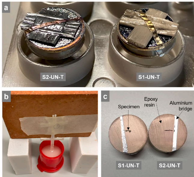
Fig. 4. SEM sample preparation: (a) samples to be analysed in top view, (b, c) samples to be analysed in cross section, by embedding them in epoxy resin (b) to obtain the final samples (c).
