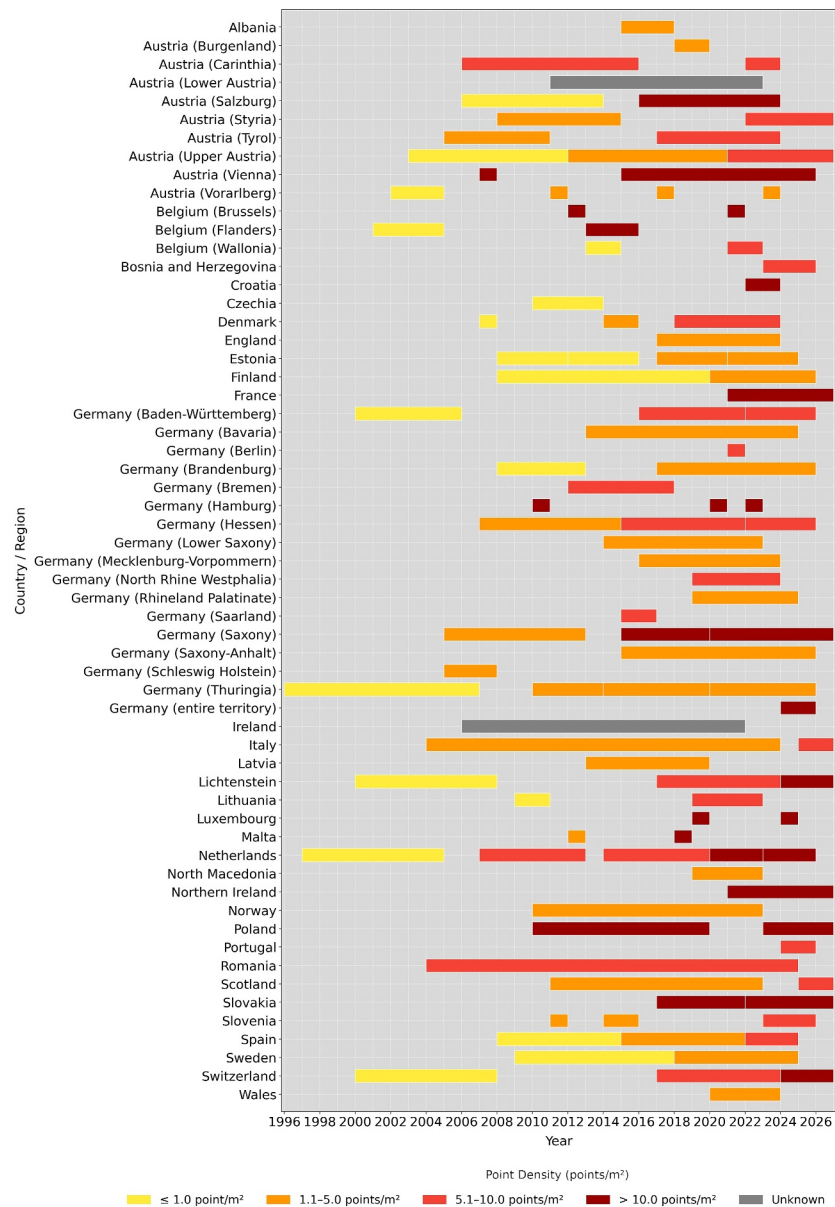
Figure 3. Years of acquisition of airborne laser scanning campaigns conducted by governmental institutions in Europe, including point density information where available. Note that the information provided is likely incomplete, both in terms of available data and their metadata, as these are documented to varying degrees and reliability. In addition, the years of acquisition may also include the preparation and processing time (i.e., \pm 1 year), as it is often difficult to distinguish whether only the acquisition years are reported or if they also include data processing. Similarly, it is difficult to distinguish whether point or pulse density is reported, and whether these are nominal/minimal densities or realized densities (which are often higher). Therefore, we use the single term point density.
