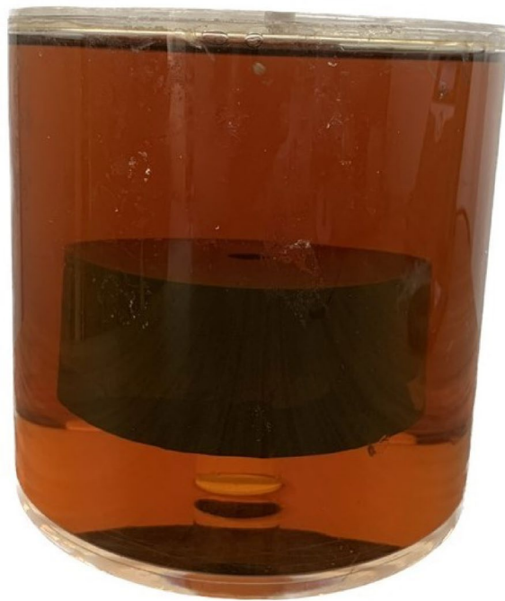
Fig. 5. The phantom is composed of a fiber ring with uniform anisotropy at each position, which is embedded in a homogeneous medium of water and sodium chloride to mimic restricted anisotropic diffusion in brain tissue.
