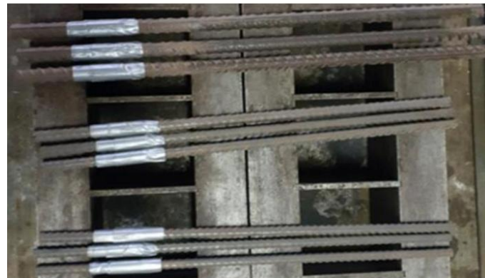
Figure 4. Surface deformation of steel bars.
