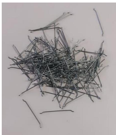
Figure 2. Hooked-end steel fibers were used in the study.
