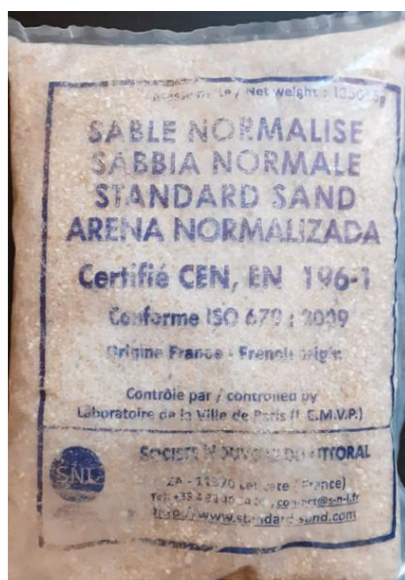
Figure 3. Sand grading conforming to EN 196-1 standard [37].
