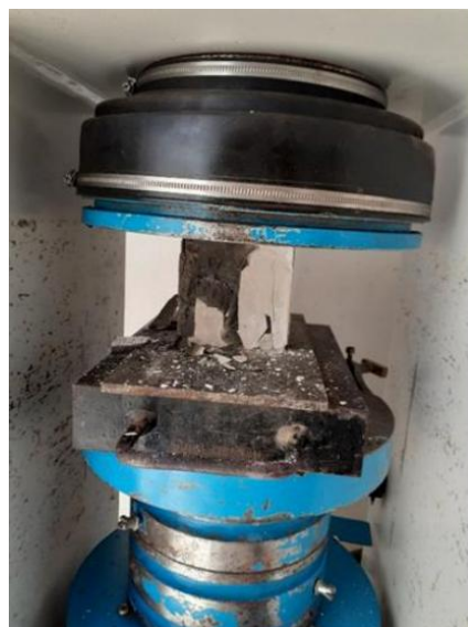
Figure 8. Sample in the compression testing machine.
