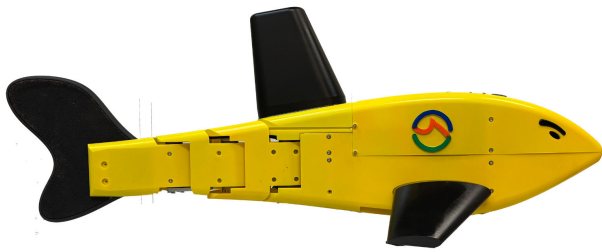
FIGURE 1. The external structure and biomimetic design of Poseidrone, the underwater robotic fish.
