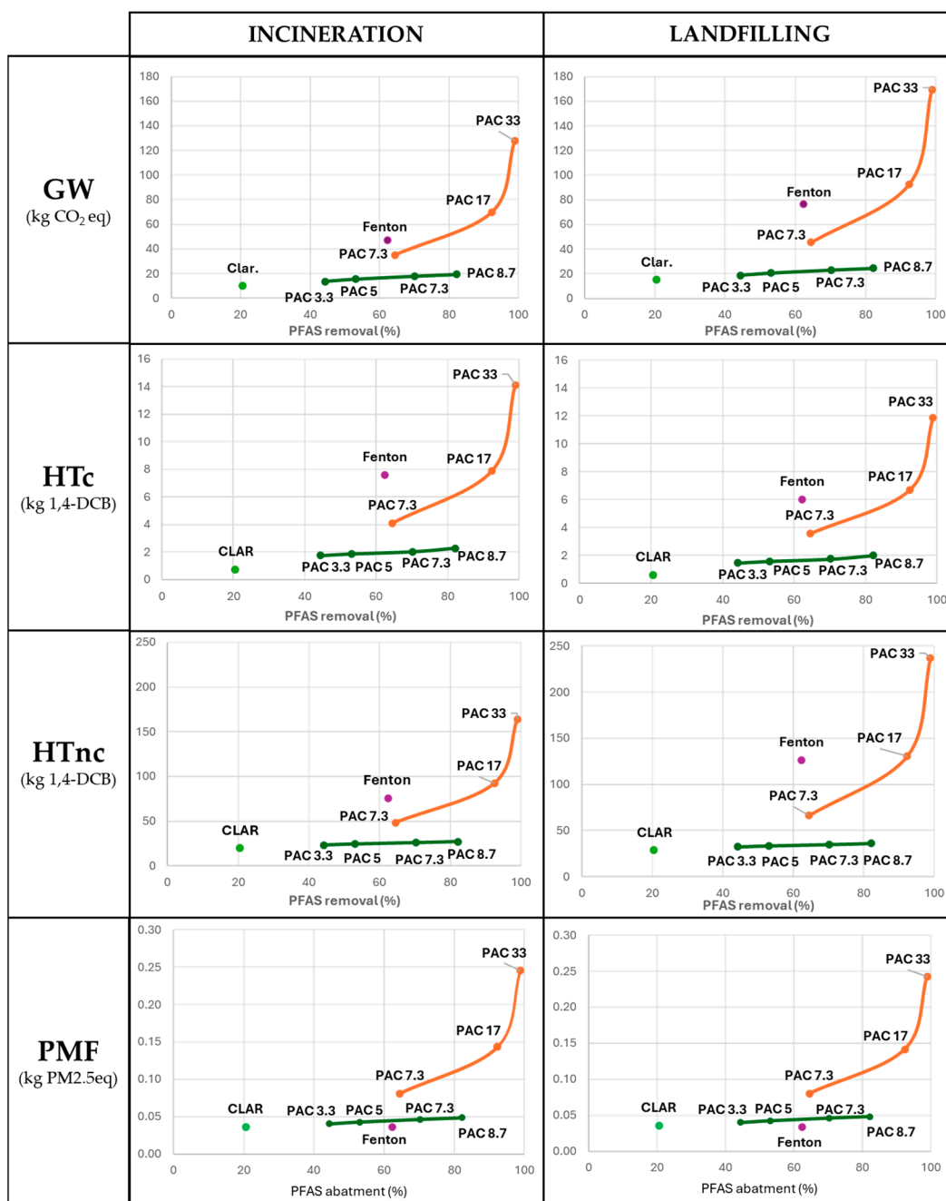
Figure 3. Results on global warming (GW), human carcinogenic toxicity (HTc), human non-carcinogenic toxicity (HTnc), and particulate matter formation (PMF) obtained according to the treatment of 1 m 3 of leachate as FU and correlated to the PFAS removal efficiency (%) for each technique. The results are presented in two columns, representing the two possible end-of-life pathways for the sludge: incineration on the left and landfilling on the right. The orange line links and highlights the trend followed by the PAC SS (single-step) processes. The green line follows the trend set by the PAC DS (double-step) processes.
