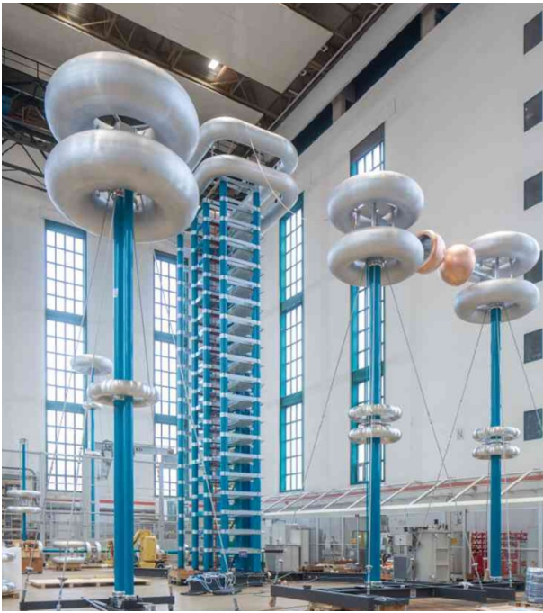
FIGURE 7 | TOV system with an extra large capacitance impulse system and spark gap (Courtesy HIGHVOLT Prüftechnik Dresden GmbH, Germany).
