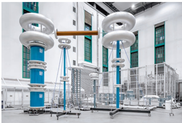
FIGURE 4 | Modular HVDC test generator system providing a total output voltage of 1.2 MV-DC (Courtesy HIGHVOLT Prüftechnik Dresden GmbH, Germany) [72].
